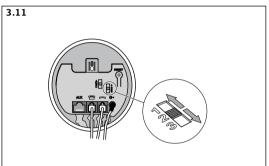
**3.11** Adjust outgoing volume with transmit volume control on base unit. Switch through the 3 settings until test person confirms the appropriate volume. <sup>1)</sup>
